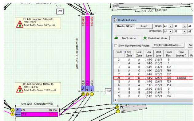
Figure 10. Additional Lane Connectors added, flows manually entered and locked. Degree of saturation balanced.
